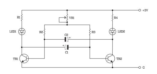
Figure 2. JUMBO 2 LED FLASHER circuit
