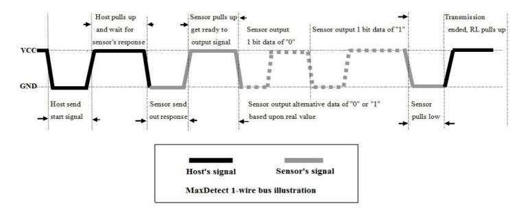
1) Step 1: MCU send out start signal to RHT03 and RHT03 send response signal to MCU
