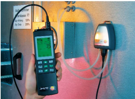
Precision measuring instrument for all pressure ranges: Differential pressure measurement at a filter with external pressure probe
