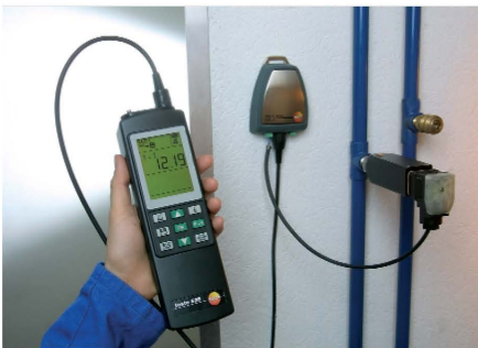
Precision measuring instrument for any parameters: Testing a transmitter with 0/4 ... 20 mA interface
