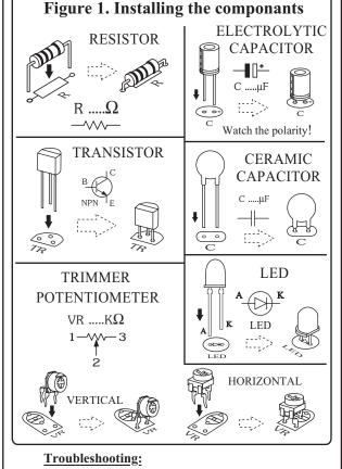
The most problem like the fault soldering. Check all the soldering joint suspicious. If you discover the short track or the short soldering joint, re-solder at that point and check other the soldering joint. Check the position of all component on the PCB. See that there are no components missing or inserted in the wrong places. Make sure that all the polarised components have been soldered the right way round.
