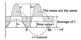
The rms value (effective value) is the DC value that generates the same thermal action as the alternating current. With I as the DC value that produces the same thermal action as the alternating current:
