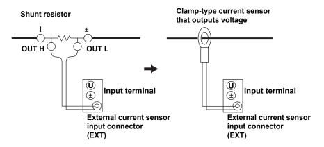
The assignment of elements to the input terminals in the figures below varies depending on the number of installed input elements. For details, see "Number of Installed Input Elements and Wiring Systems" in section 2.3, "Measurement Conditions."
