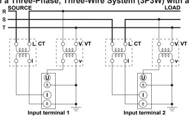
Wiring Example of a Three-Phase, Three-Wire System with a Three-Voltage, Three-Current Method (3P3W; 3V3A), a VT, and a CT
