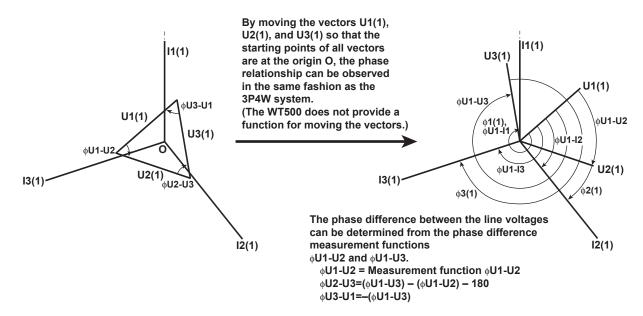
Vector Display When the Wiring System Is 3P3W (Three-phase, three-wire) U1(1), U2(1), and U3(1) are line voltages. I1(1), I2(1), and I3(1) are line currents. However, U3(1) and I3(1) are not actually measured for the 3P3W system. The vectors are displayed through computation.
