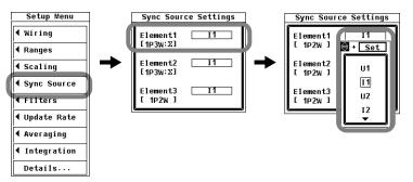
The measurement period is determined by the data update rate (see section 4.9 for details) and by the synchronization source, which is specified by following the procedure described in this section. For details, see appendix 6.
