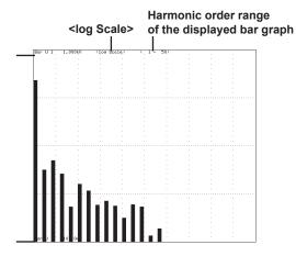
U or I, for voltage or current; the element number; and the lower limit of the displayed bar graph
