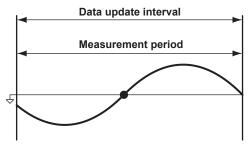
Because of the reasons described above, the measured voltage and current values may be unstable. If this happens, lower the data update rate so that more periods of the input signal fit within the data update interval.
