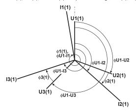
• Vector Display When the Wiring System Is 3P3W (3V3A; Three-voltage, three-current) U1(1), U2(1), and U3(1) are line voltages. I1(1), I2(1), and I3(1) are line currents.
