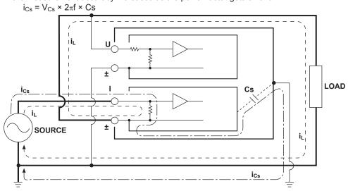
Because the WT500 measures high frequencies, the effects of  $i_{Cs}$  cannot be ignored. If you connect the WT500 current input terminal to the side that is close to the earth potential of the power source (SOURCE), the WT500 current measurement circuit positive and negative terminals are close to the earth potential, so  $V_{Cs}$  becomes approximately zero and very little  $i_{Cs}$  flows. This reduces the effect on measurement accuracy.
