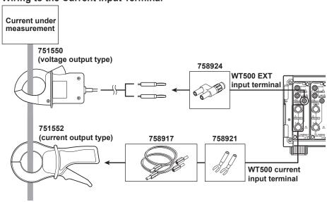
Connecting a clamp-on probe
