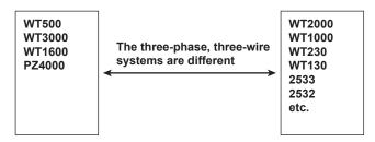
For example, if you replace the WT2000 (used in a three-phase, three-wire system) with the WT500 and leave the wiring unchanged, the measured power of each element will be different between the WT2000 and the WT500. Refer to this manual and re-wire the system correctly.
