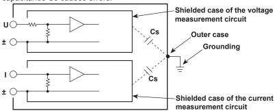
As an example, we will consider the case when the outer case and one side of the power source are grounded.
