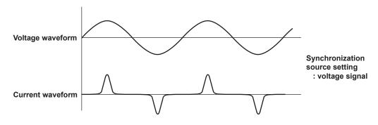
As another example, if an inverter is being measured and the distortion of current waveforms is smaller than voltage waveforms, set the synchronization source to the current signal.
