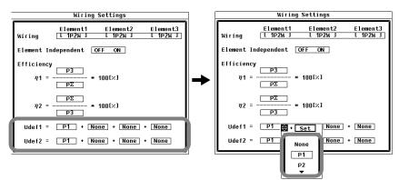
You can create an efficiency equation can by combining measurement function symbols. The WT500 can determine the energy conversion efficiency of the device using the numeric values of the measurement functions.
