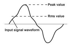
The crest factor on the WT500 is determined by the ratio of the maximum peak value that can be applied for rated input to the measurement range.
