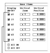
Indicators that tell whether the waveform displays of each input signal are on or off
