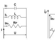
The relationship between resistance  $R_P$ , reactance  $X_P$ , and impedance Z is expressed by the equations below.
