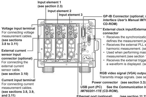
GP-IB Connector (optional; see the Communication Interface User's Manual IM760201-17E on the
