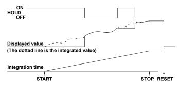
If you stop integration while the display is held, the displayed and transmitted values do not change. When you release the hold function (turn it off) or make a single measurement by pressing SHIFT+HOLD (SINGLE), the integration result at the point when integration was stopped is displayed or transmitted.
