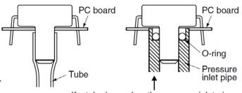
If a tube is used as the pressure inlet pipe, it may become disengaged. Therefore, use a sturdy tube and secure it using O-rings.
