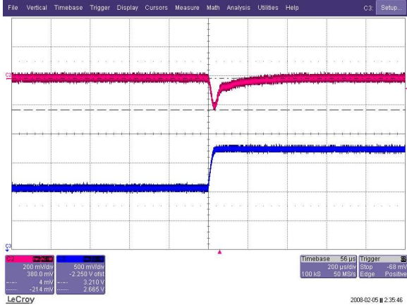
[Fig.22] Load step: 50%-75% of I_o , di/dt=0.1A/\mu s (CH1: 200mV, CH2: 2.5A/div, 200us/div)
