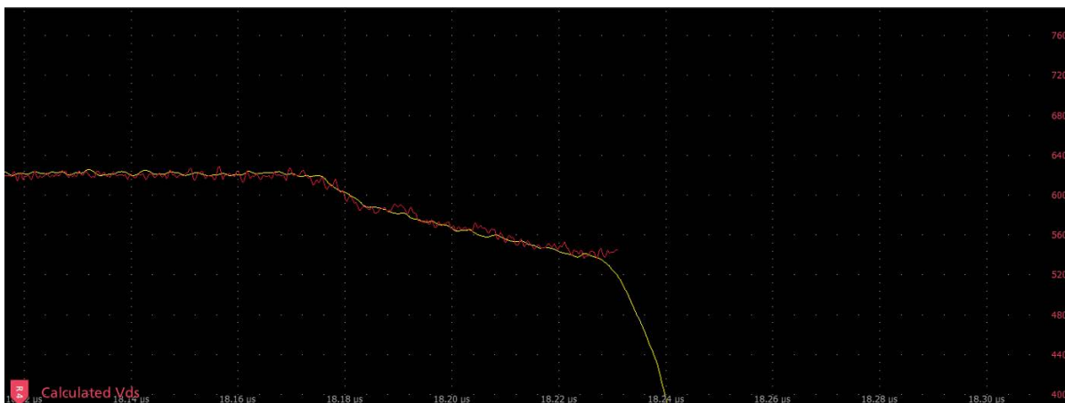
Figure 39: V_{ds} modeled using perfectly differential order of filter at turn on transient
