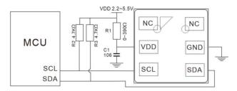
Figure 15. Typical Application Circuit
