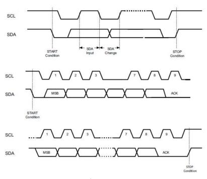
Figure 17. I<sup>2</sup>C bus timing diagram
