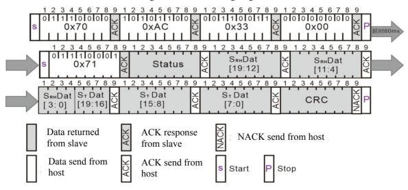
$0x70\ 0xAC\ 0x33\ 0x00$  is to send the write measurement command byte segment to the sensor;
