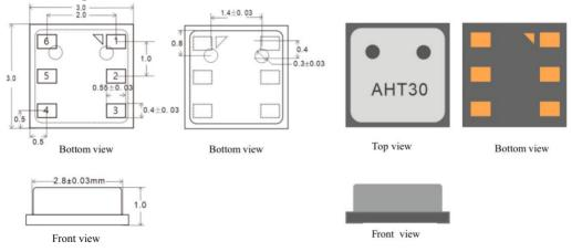
Figure 1: AHT30 temperature and humidity sensor (Unit: mm Tolerance: ±0.1 mm)
