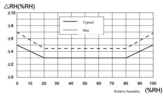
Figure 2. The typical error and Max error of Relative humidity at 25°C
