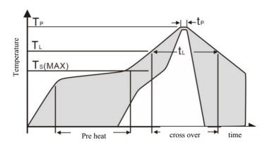
Figure 9. JEDEC standard soldering process diagram,  $T_P < 200\,^{\circ}\text{C}$ ,  $t_P < 30\text{sec}$ , lead-free soldering.  $T_L < 180\,^{\circ}\text{C}$ ,  $t_L < 150\text{sec}$ , and the rate of temperature rise and fall during soldering should be  $< 5\,^{\circ}\text{C/sec}$ .
