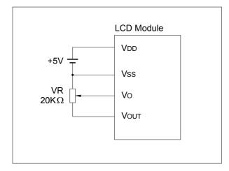
VO is LCD driving voltage (contrast adjusting). Adjust VDD-VO to be around 12.7V for the best contrast.
