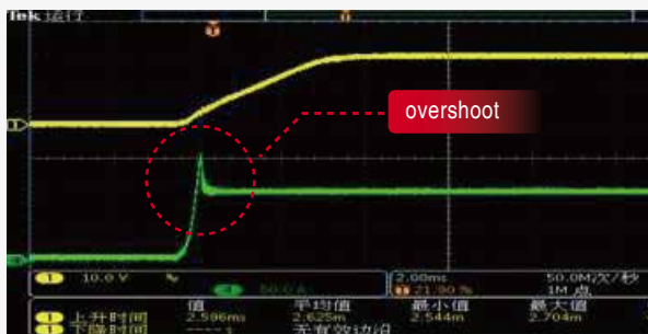
Diode load Conventional power test
