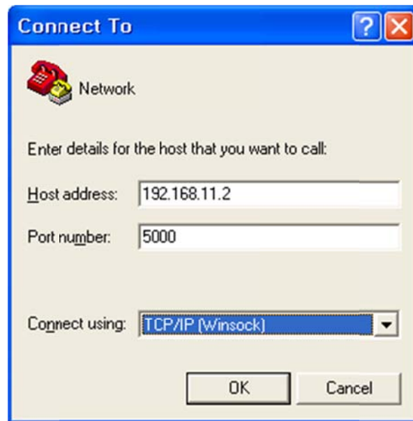
Figure 24. Network Terminal Program configuration
