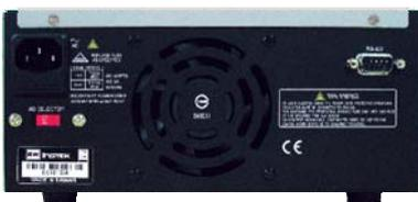
The PSP-Series is single output, 200W, programmable switching DC power supplies. OVL, OCL, OTP, and OPL protect the PSP-Series and its loads from unexpected conditions. The PSP-Series has a large LCD panel with output and parameter views and a key lock feature to prevent changing the settings. The PSP-Series is suitable for generic bench-top applications in laboratories and educational institutions.
