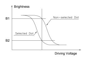
Contrast Ratio =  $\frac{\text{Brightness of non-selected dot (B1)}}{\text{Brightness of selected dot (B2)}}$
