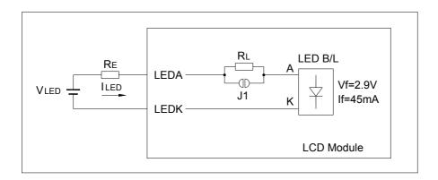
RL (internal) and RE (external) are the current limiting resistors for LED backlight
