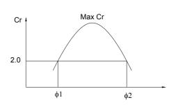
Note2: Definition of viewing angle range  $\phi 1,\, \phi 2$
