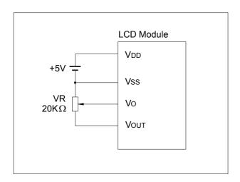
VO is LCD driving voltage (contrast adjusting). Adjust VDD-VO to be around 11.2V for better contrast.
