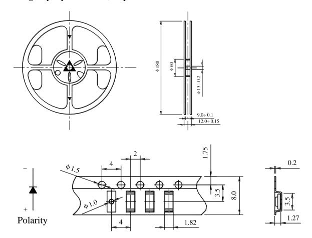
Reel Lead Min.60mm No LEDs
