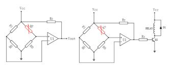
This is an ideal circuit for applications that require on-off switching at a specified force. It consists a Wheatstone bridge circuit and a voltage comparator.
