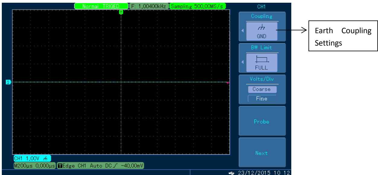
Fig. 2-4 Both the AC and DC Components in a Signal have been blocked Simultaneously
