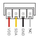
Figure 4 CM2122 Wiring Diagram
