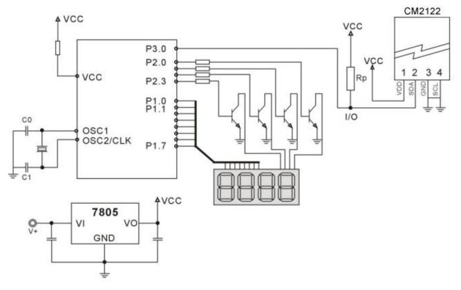
Figure 4 CM2122 One-Wire Application Circuitry
