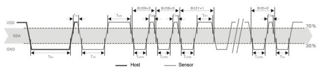
Figure 6 CM2122 Single bus communication timing
