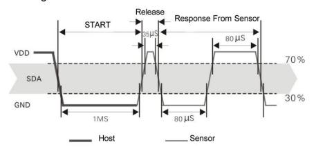
Figure 7 Single Bus Decomposition Timing Diagram
