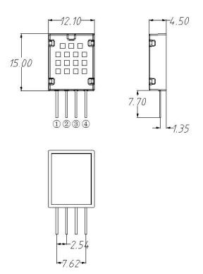
**Figure 1** Dimension (Units: mm) **Pins** 1 VDD 2 SDA 3 GND 4 NC
