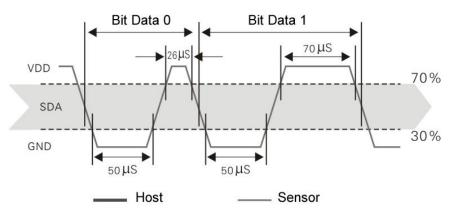
Figure 8 Single Bus Decomposition Sequence Diagram
