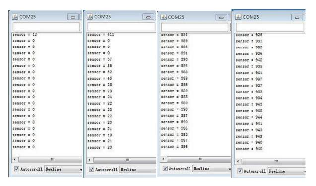
Sensor in air Sensor in dry soil Sensor in humid soil Sensor in water
