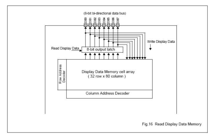
The setting of the control bus for issuing Read Display Command
