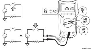
Figure 2. Measuring AC and DC Current
