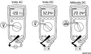
Figure 1. Measuring AC and DC Voltage
