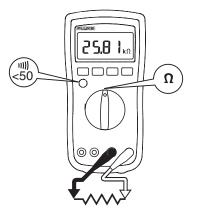
Figure 3. Measuring Resistance/Continuity
