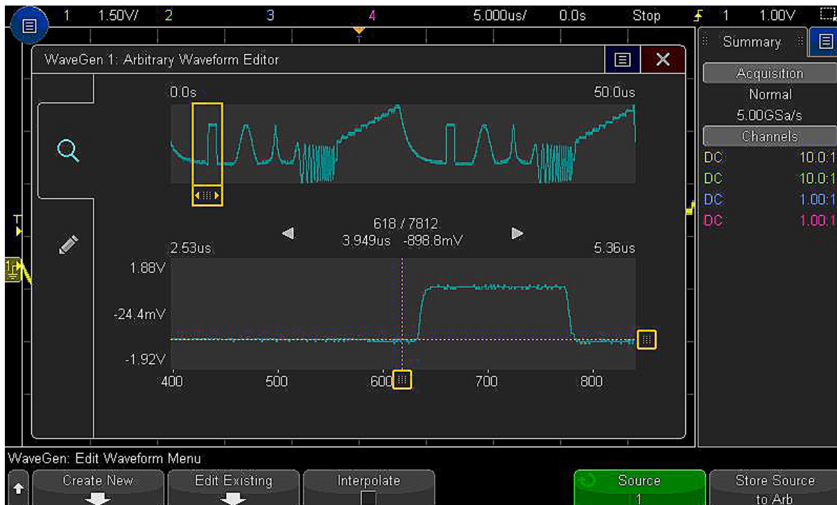
Figure 29. Standard arbitrary waveform generator provides easy access to stimulus. The integrated arbitrary waveform generator makes capturing, modifying, and replaying signals simple.
