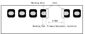
Note: There is a slot(non-metallic hole) between pin 4/5, which the side pad were being cut off. For details, please refer to the recommended dimensions or pad.
