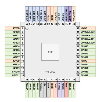
GPIOx General-purpose digital input and output
