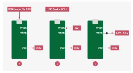
There are three main ways we can safely power Raspberry Pi Pico, and the choice is entirely dependent on your application. We can either power Raspberry Pi Pico from the **micro USB connector** on the device itself (option (a) in Figure 13), or we can provide power to either the **VBUS pin** (option b), or the **VSYS pin** (option c).
