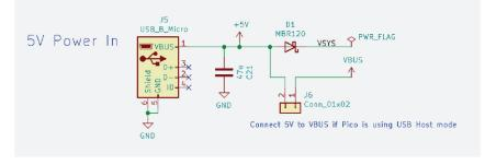
The **VSYS pin** is the main system power supply on Raspberry Pi Pico. From this supply, Raspberry Pi Pico generates its own 3.3V supply which is used to power RP2040, and also the 3V3 output pin of Raspberry Pi Pico which we can use to power circuits on our design.
