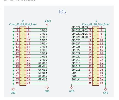
In addition to the USB connector already mentioned, there are a pair of 2x18-way 2.54mm headers (**J3** and **J4** in Figure 10), one on each side of the board, to which the rest of the IO have been connected. As this is a general purpose design,
