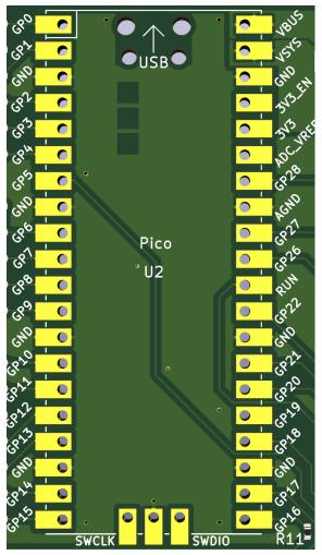
The CAD footprint provided with this design provides both options, so Raspberry Pi Pico can either be soldered direct to this design, or 0.1" headers may be used (or indeed, a combination of 0.1" headers and sockets) to connect the two PCBs together.
