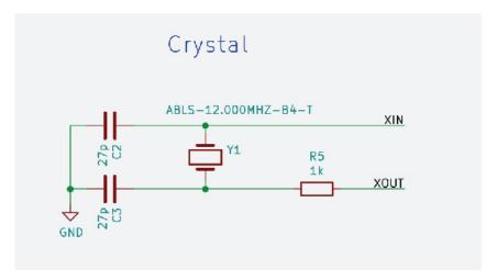
Strictly speaking, RP2040 does not actually require an external clock source, as it has its own internal oscillator. However, as the frequency of this internal oscillator is not well defined or controlled, varying from chip to chip, as well as with different supply voltages and temperatures, it is recommended to use a stable external frequency source. Applications which rely on exact frequencies are not possible without an external frequency source, USB being a prime example.
