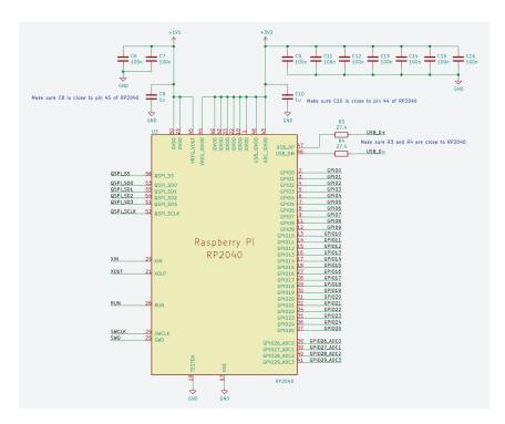
This design consists of four main elements: **power, flash storage, crystal oscillator, and IOs (Input/Outputs)**, and we'll consider each in turn below.
