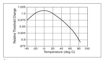
FIGURE 1. Normalized threshold irradiance vs. amb. temp.
