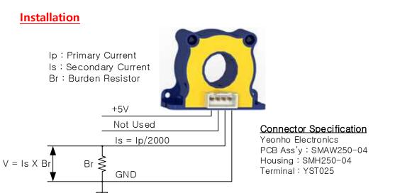
\* The positive direction of the current from the front to the rear of the head (the front of the contactor).
