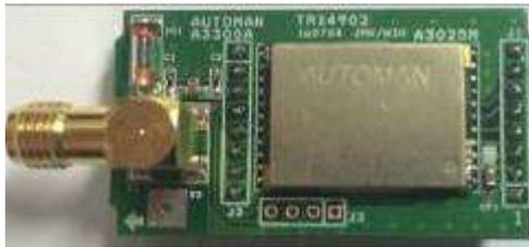
Figure 1. A3300A, 420 - 525 MHz (G)FSK modem.
